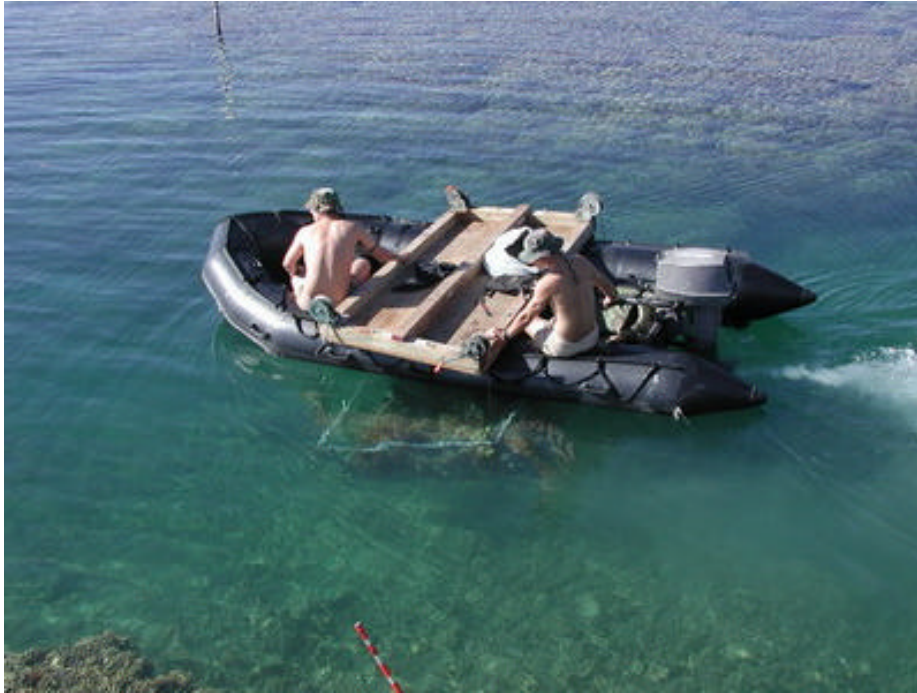
Figure 2. Moving corals from channel to patch reef using basket slung under boat with winch system used to lower or raise basket.
